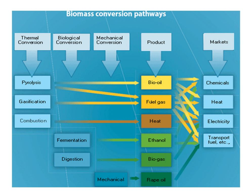
Biomass Gasification is the process of conversion of *solid* biomass to *gaseous* form by partial pyrolysis, oxidation and reduction under sub-stoichiometric conditions.
